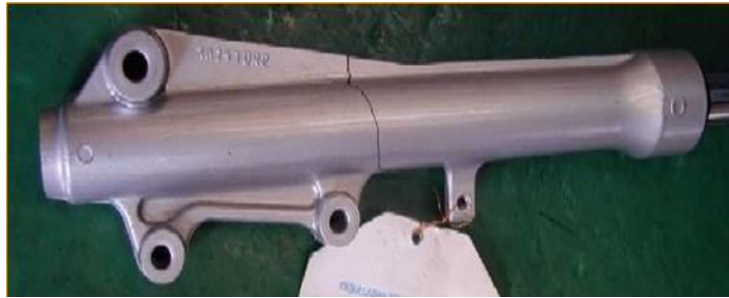
Figure 1. Crack on Tube Outer
