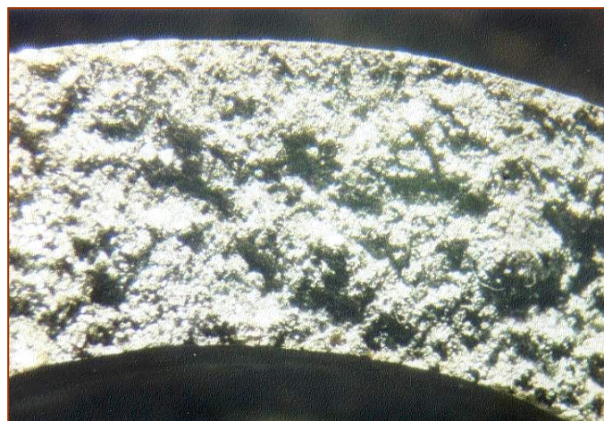
Figure 2a. Concave-Bulges Morphology on Fracture Surface (mag. 6x)
