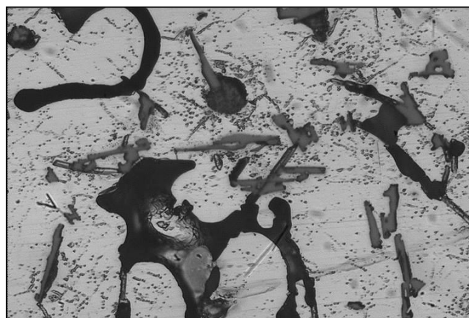
Figure 3c. Outer Tube Microstructure (visible eutectic phase and porosity between the aluminum matrix, mag. 550x)
